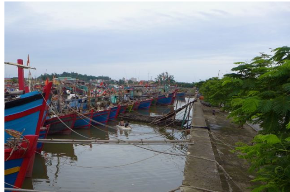
Photo 6.7 Prevention measures to protect boats by strapping to trees along embankment at Do Son area
