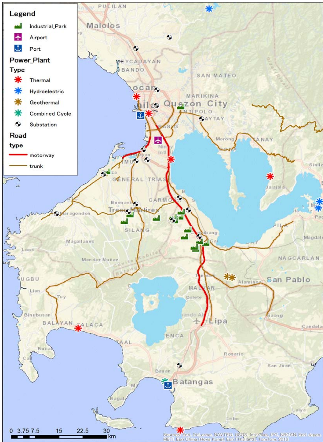
Fig.3- 1 Infrastructure facilities in the area
