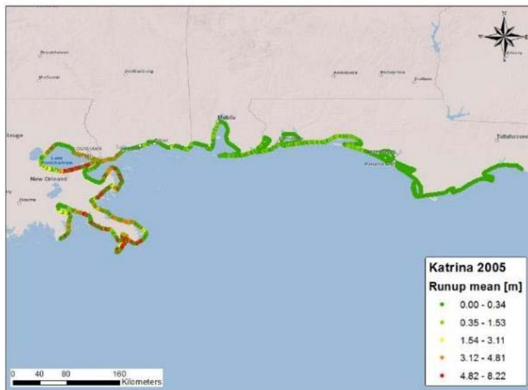
Figure 69. Mean value of the storm surge run-up along the coast of USA for 100 simulations of hurricane Katrina (2005).
