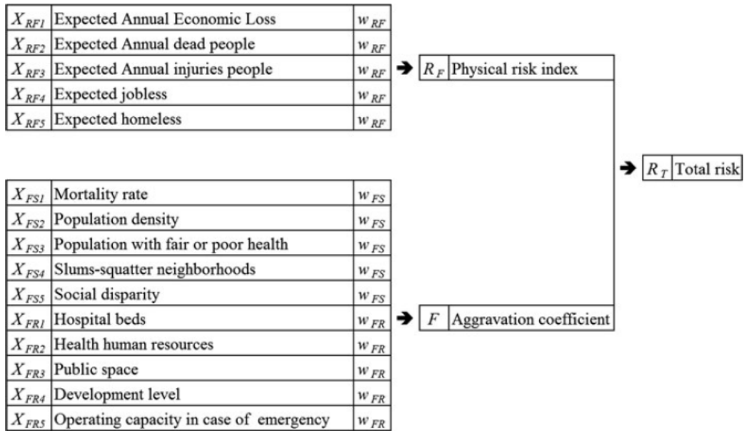
Figure A16-7. Descriptors used for the physical risk and aggravating coefficient indexes
