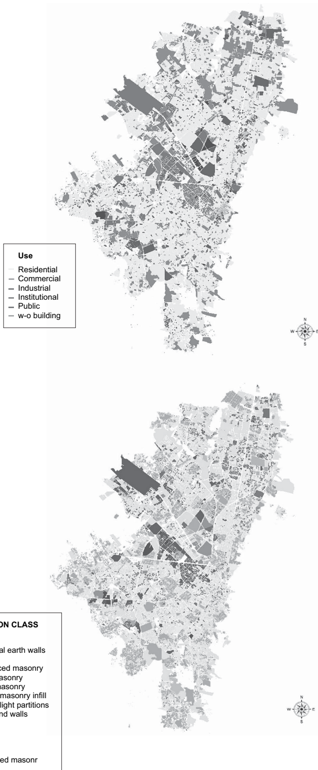
FIGURE 3 Index maps of number of stories and structural class distribution for Bogotá.
